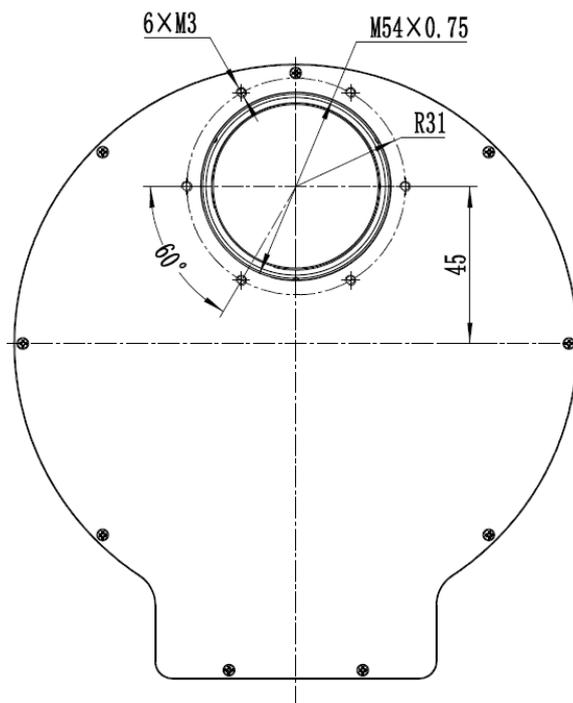
Figure 3 Back face of AFW (to telescope)
