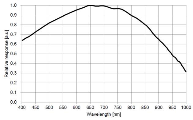
Figure 1 IMX462 Spectral Sensitivity Characteristic
