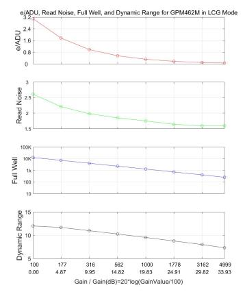
Figure 2 e/ADU, Read Noise, Full Well and Dynamic Range for GPM462M
